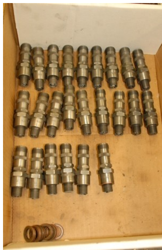
Clean and shiny spark plugs ready for installation in the Hurricane's Merlin.
